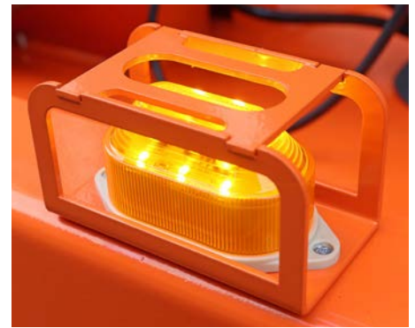
Dual flashing beacons alert pedestrians during operation.
