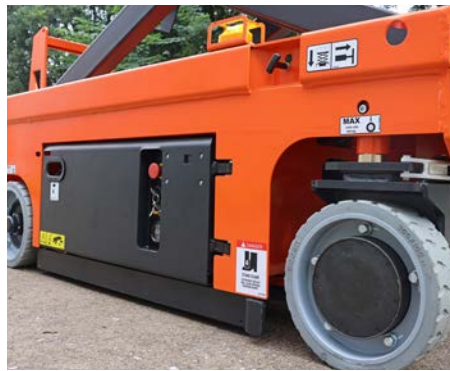
Pothole protection system automatically engages while operating in a lifted position.
