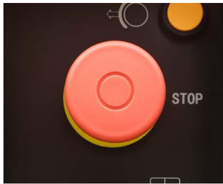
Emergency stop buttons at both platform and ground controls.
