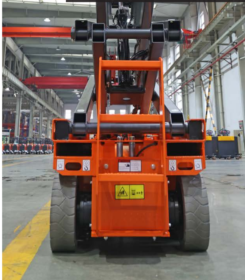
Full height travel is convenient and greatly improves productivity. Traveling speed automatically slows down in a lifted position to ensure safe operation.
