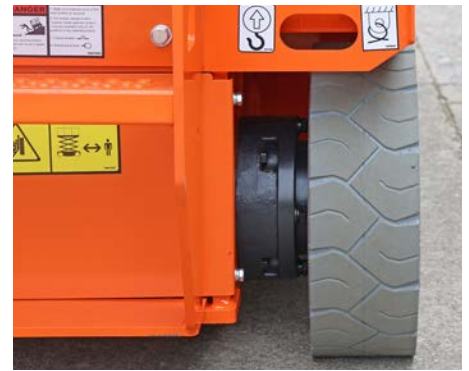
Front wheel hydraulic dynamic braking eliminates sliding while working on slopes.
